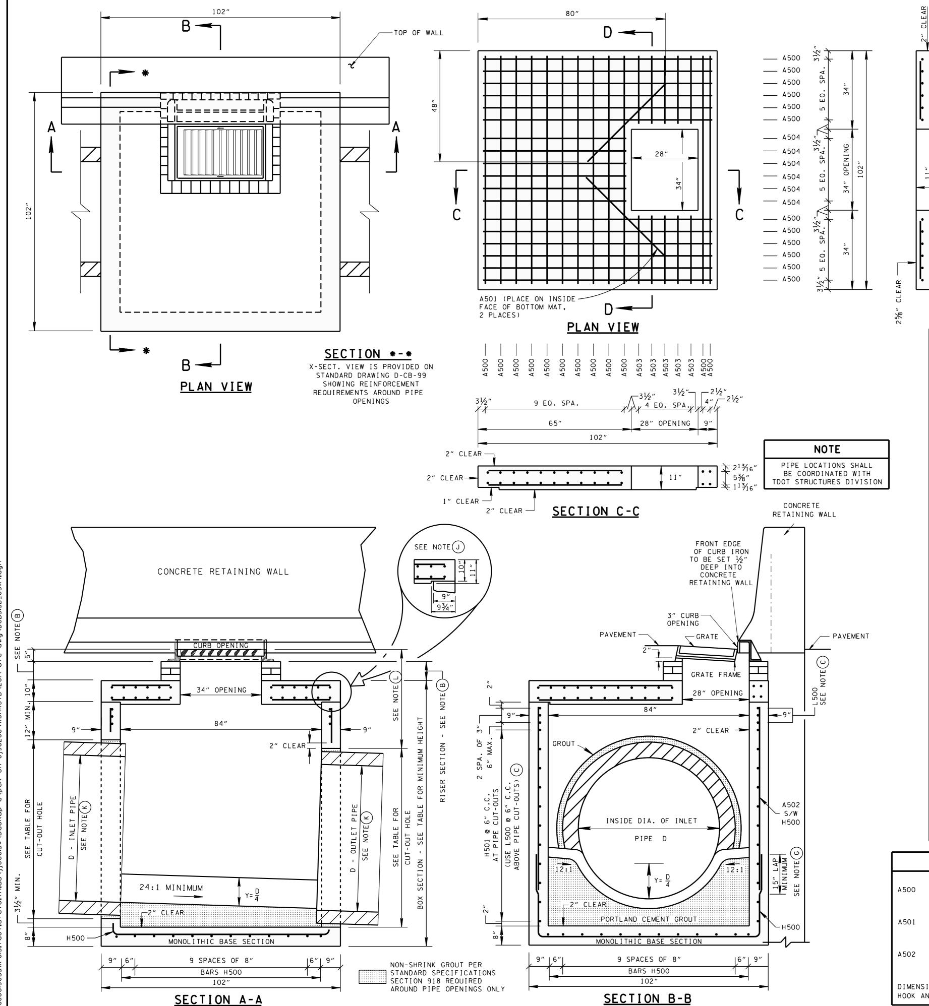
FOR DESIGN CATCH BASIN DIMENSIONS USE ONLY CATCH BASIN DIAMETER OF CUT-OUT MINIMUM MINIMUM THICKNESS (D) OF PIPE HEIGHTS DESIGN DEPTH HOLES (INCHES) (INCHES) (INCHES) (INCHES) (FEET)  $2\frac{1}{2}$ 25 4.34 32 24 641/2 4.88 39  $71\frac{1}{2}$ 5.42 46 5.97 78½ 53 6.51 60 7.05 51/2 67 991/2 7.59 74 1061/2 8.13  $113\frac{1}{2}$ 8.67 81
